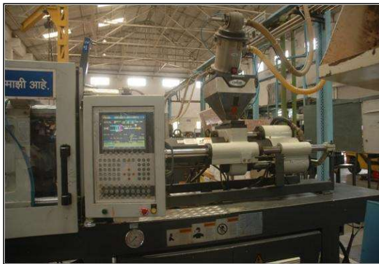
INJECTION MOULDING (110 T – 350 T)
